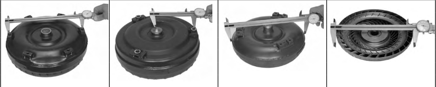
Bolt Circle Center of Pad to Center of Pad Bolt Radius (x 2 = Bolt Circle) Center of Pad to Center of Pilot Diameter - Overall Outside of Conv. (Not Ring Gear) Diameter - Turbine Outside of Turbine (Internal)
