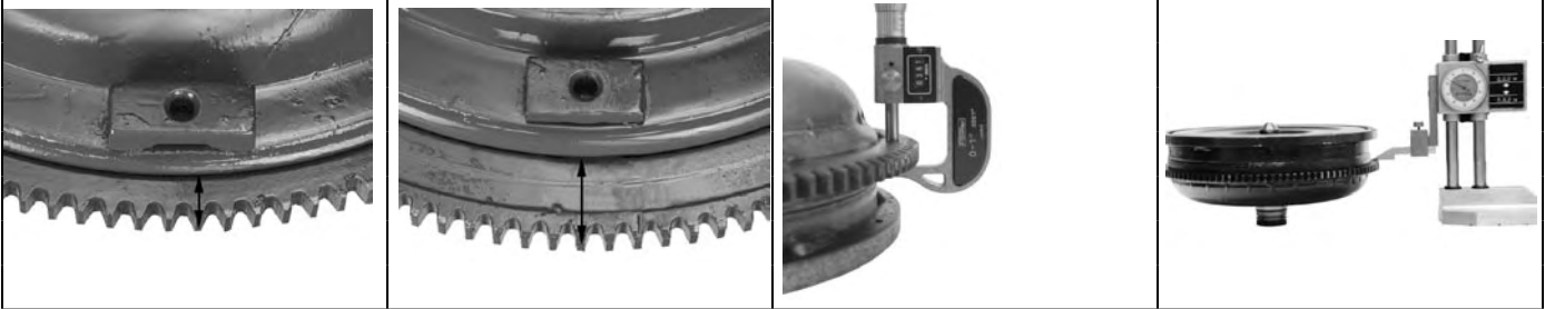
Ring Gear (Narrow) Converter to Outside of Gear Ring Gear (Wide) Converter to Outside of Gear Ring Gear Thickness Thickness of Gear Ring Gear Height Top of Gear to Top of Hub
