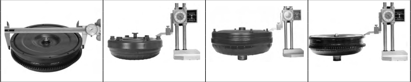
Mounting Ring - Outer Outside of Ring to Outside of Ring Overall Height w/ Pads Top of Pad to Top of Hub Overall Height w/ Studs Top of Stud Base to Top of Hub Overall Height w/ Ring Top of Mounting Ring to Top of Hub
