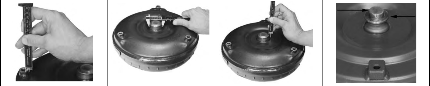
Pad Height Outside of Pad to Converter Pilot Diameter Outside of Pilot Pilot Height Top of Pilot to Top of Hub Pilot Stepped Measure Both Steps
